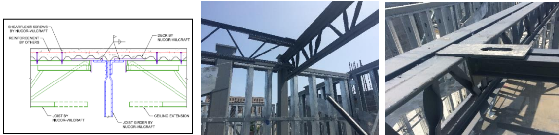
Figure 5. Ecospan® Flush Bearing Seat-to-Joist Girder Connection
